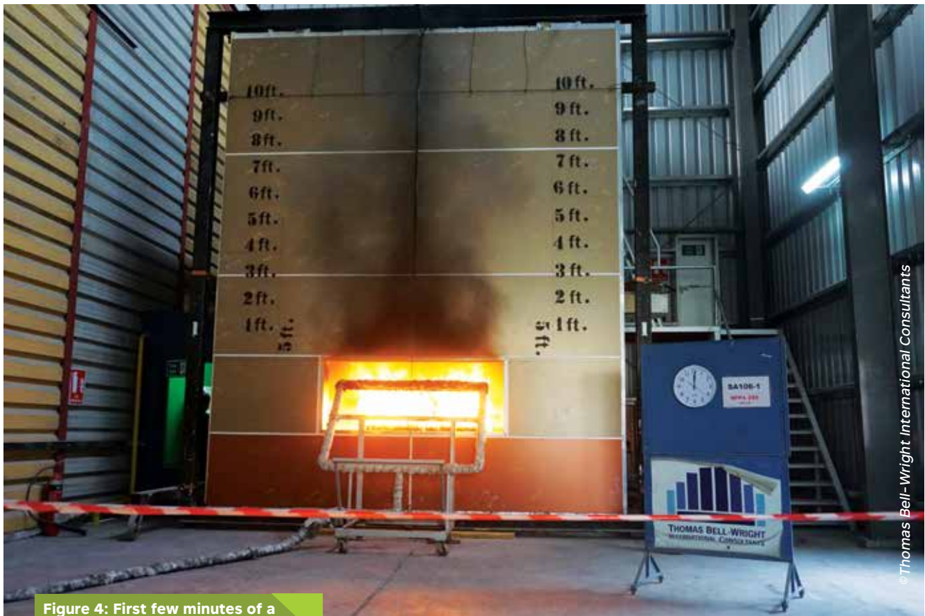
Figure 4: First few minutes of a test where mock-up has joints
