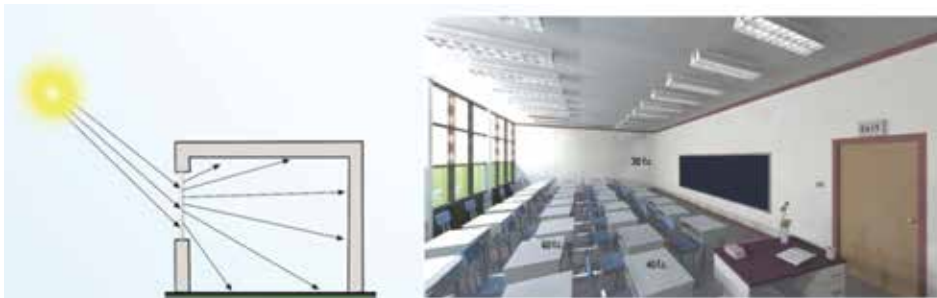
Solera aerogel infilled glasses scatter the light flowing through it evenly across the room
