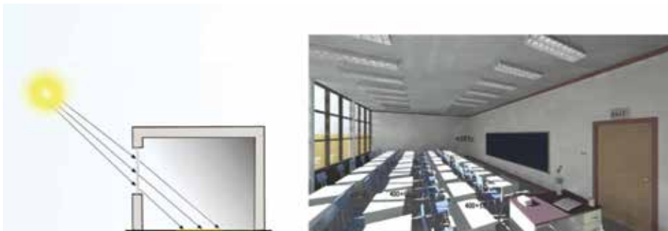
Conventional glass windows are not light diffusing and allow light to pass in straight lines
