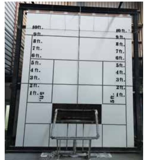
A test construction ready to undergo fire testing to NFPA 285
