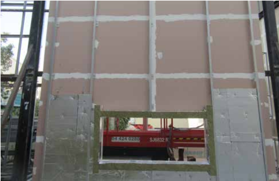
Picture 2: one of several typical ways used to protect the window opening facing a unique fire situation created during the fire test
