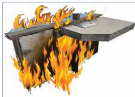
Resistance to fire test on spandrel panel assembly
