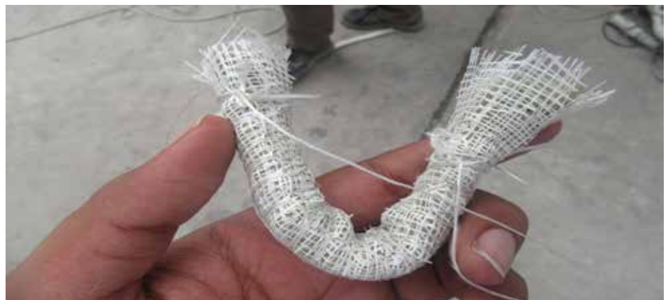
Picture 3: Contractors fill the panel joint gaps with fire rated backer rods for the mock-up of the tests
