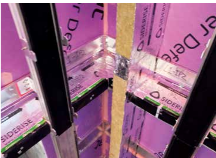
Siderise has participated in and sponsored many large-scale system tests where the test assembly uses their RH and RV Cavity Barriers and CH-CB Closed State Horizontal Cavity Barriers
